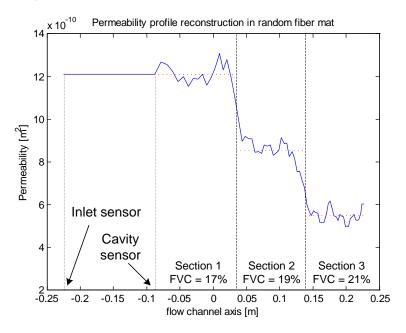
Figure 1: Permeability reconstruction during the impregnation of a random fiber mat preform with three FVC sections.
